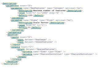
Fig. 3: The CAVIAR description for the DenseImageFeatures module.
