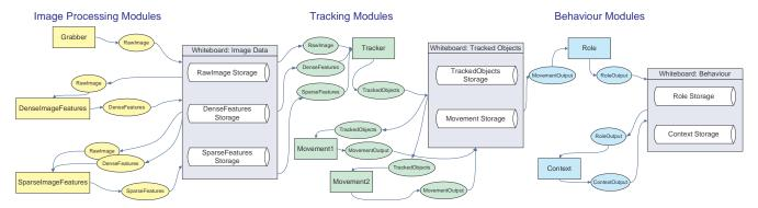
Fig. 2. The system data and processing flowchart from Psyclone. (Data structures are listed twice, once for input and once for output.)
