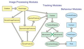
Fig. 1. The system data and processing flowchart from CAVIAR
